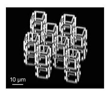
Fluorescence imaging of a silver nanostructure created with ImpFab. Credit: *Science*.
