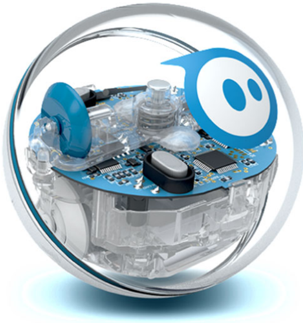
Fig. 2. Sphero (a generic SRR). Picture source: http://www.sphero.com/sphero .
