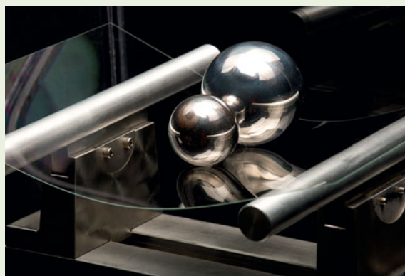
A piece of Corning’s Gorilla Glass undergoing a flexibility test in the laboratory. Image courtesy of Corning Incorporated.
