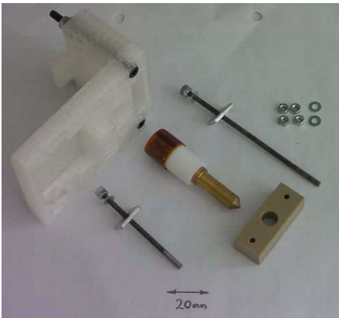
Fig. 9. The latest standard RepRap nozzle design partly disassembled. The PTFE ends in a narrow section that screws inside the brass. The PEEK bracket is the part with three holes. The brown material at the top of the PTFE is Kapton tape to ensure a snug fit in the extruder transport mechanism.
