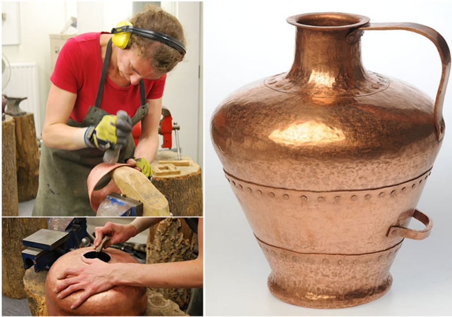
5.2. Upper left: Clarke raising the top section/neck of the copper hydria using a wooden stake and granite pestle. Lower left: using a fine-grained sedimentary stone to grind down sharp edges left after cutting a hole in the shoulder section with a chisel. Right: copper hydria modelled after a bronze Late Minoan IIIA1 hydria in the Archaeological Museum of Chania; 44cm high. © Upper and lower left: C. Clarke (photo by Lan Nguyen-hoan); right: C. Clarke (photo by J. Kuhnen).
