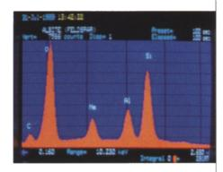
High sensitivity elemental analysis is possible with the addition of an EDS system.
