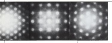
High resolution, electron microdiffraction analysis may require several tilt angles.
